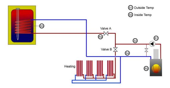
Two port valves offer easy to understand wiring.
