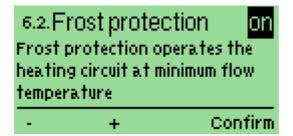
The heating pump (R1) is activated if the outside temperature is less than 1C.
