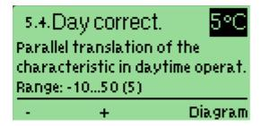
A default level of 5  $^{\circ}$ C is added to the curves predicted output during periods when the heating timer is active. This helps increase the heating response time. This helps the heating response time.
