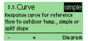
A simple or split curve is used to calculate the heating circuit flow temperature target depending on the outside temperature.
