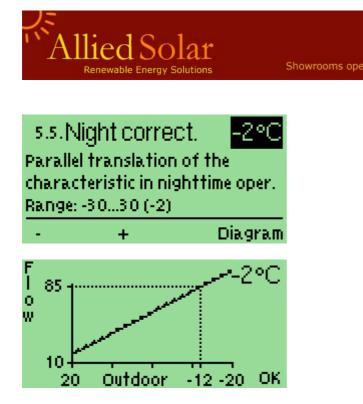
To Save energy during periods when the heating timer is not active, the curve temperature can be set-back. The Default value is 2C.
