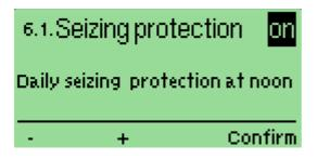
Turn on boiler pump and exercise valves at 12:00 for 5 seconds every day to prevent seizing from periods of inactivity.
