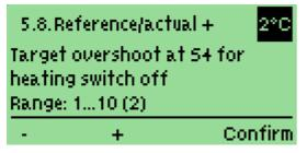
Turn boiler off (R5) when S4 temperature is above the target temperature by this amount.
