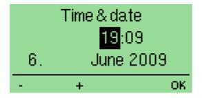
Input the time, note the time will stay accurate for 24hours if mains power is disconnected, after this period the clock must be reset.
