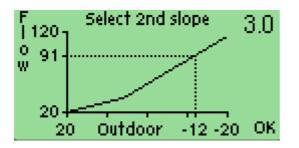
A split curve is also available. During cold weather (e.g. 6 °C or below) it is possible to change the slop of the curve so that the heating responds more aggressively below this outside temperature. This can be especially helpful in older houses with poor insulation.
