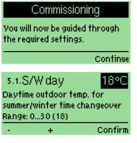
If the **heating timer** is active and the outside temperature is greater than this value, the heating circuit is deactivated.
