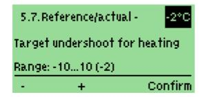
Hysteresis Negative, turn on boiler ONLY when the temperature measured at S4 is below the targeted temperature by this amount. (NOTE: there is a 5 minute delay on boiler firing to overcome boiler hunting)
