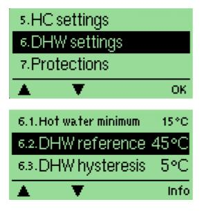
If the temperature in the cylinder drops below the "hot water minimum" then the boiler and hot water circuit is turned on regardless of the state of the timer.
